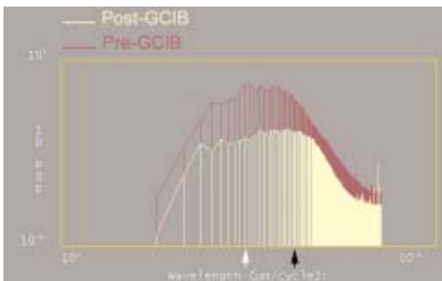
To correlate the performance of a resonator with its surface topography, Veeco AFM built-in analysis software offers a myriad of options to quantify the images. It can measure the rms roughness, identify the dominant wavelengths that contribute to the roughness, and can compare roughness before and after critical process steps at a given location or between different locations.
