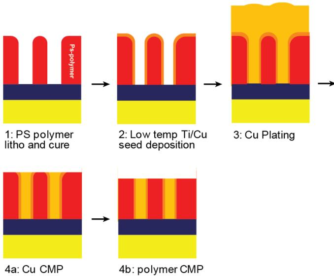
**Fig. 7:** Fabrication steps for damascene process flow. The resulting meandercomb structures are tested for electrical shorts and resistance.
