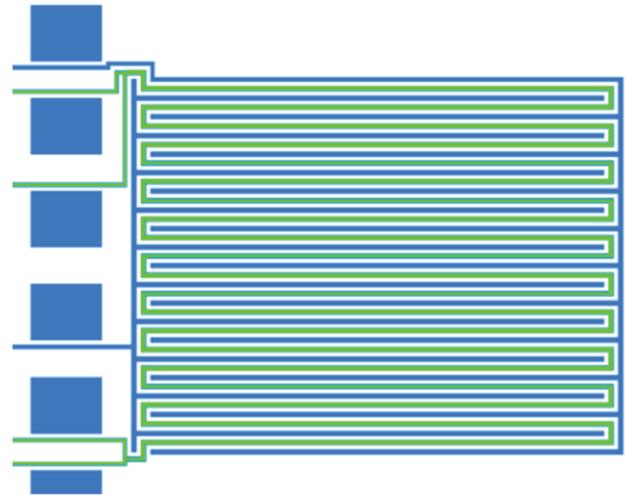
**Fig. 8:** Meandercomb structure used for electrical testing. The resistor under test is in green and the finger structure for leakage current testing is in blue.
