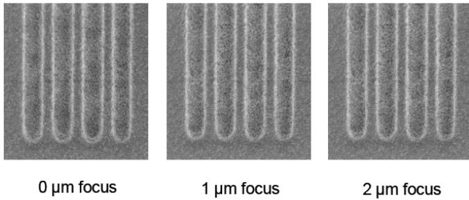
**Fig. 4:** Top down SEM images of 1.0µm line/space in 3µm thick JSR photosensitive dielectric on Si through focus, i-line exposure, 0.20 NA.
