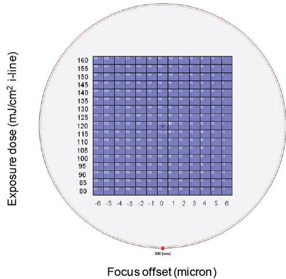
**Fig. 2:** Wafer layout for the FEM. A thirteen column by seventeen row array of fields was exposed with focus varying in the horizontal axis and exposure varying in the vertical axis.
