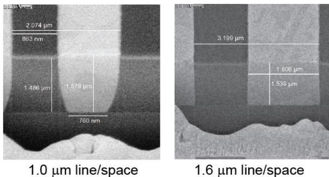
**Fig. 11:** Focus ion beam cut of 1.0 $\mu\text{m}$  and 1.6 $\mu\text{m}$  Cu lines after completing the full CMP process.
