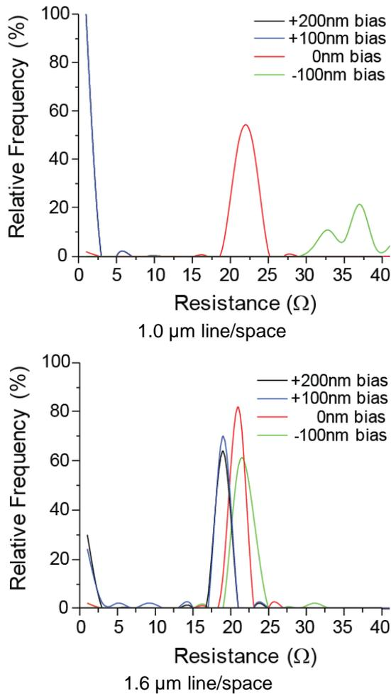
**Fig. 14:** Electrical testing in leakage mode produces high yield of 100% for 1.0 $\mu\text{m}$  line/space and 90% for 1.6 $\mu\text{m}$  line/space. The lower yield for the larger 1.6 $\mu\text{m}$  structure is attributed to accidental FIB cuts prior to electrical testing.
