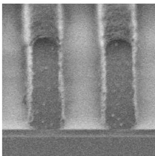
Cross sectioned 1 µm line/space
