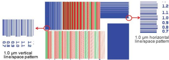
**Fig. 1:** Reticle UT678B test pattern contains a variety of line/space and square via patterns designed for SEM cross section work.
