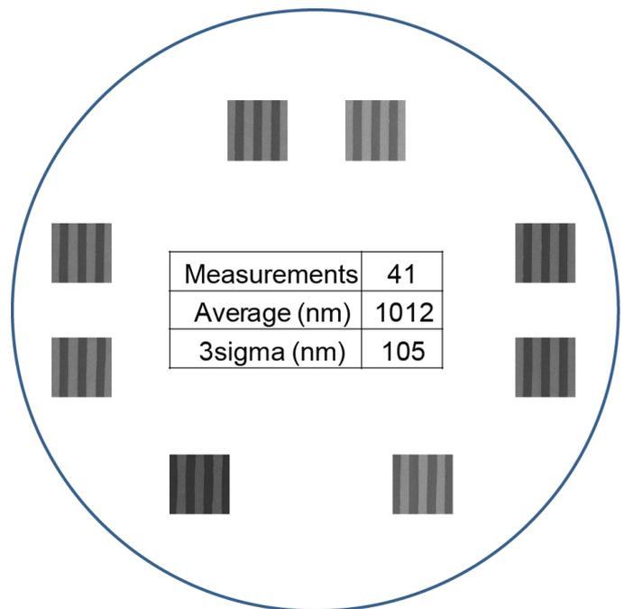
**Fig. 13:** CD of 1.0 $\mu\text{m}$  damascene lines measured at 41 points across wafer averages 1012nm with 3 $\sigma$  of 105nm.
