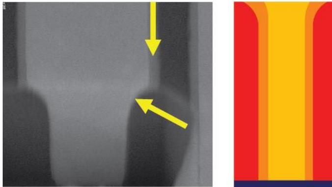
**Fig. 10:** Dielectric and Cu profile after Cu and barrier CMP. Further recess CMP is required to remove the round-off and Cu smearing. The actual image is compared with the CMP process step 4(a) shown in figure 7.
