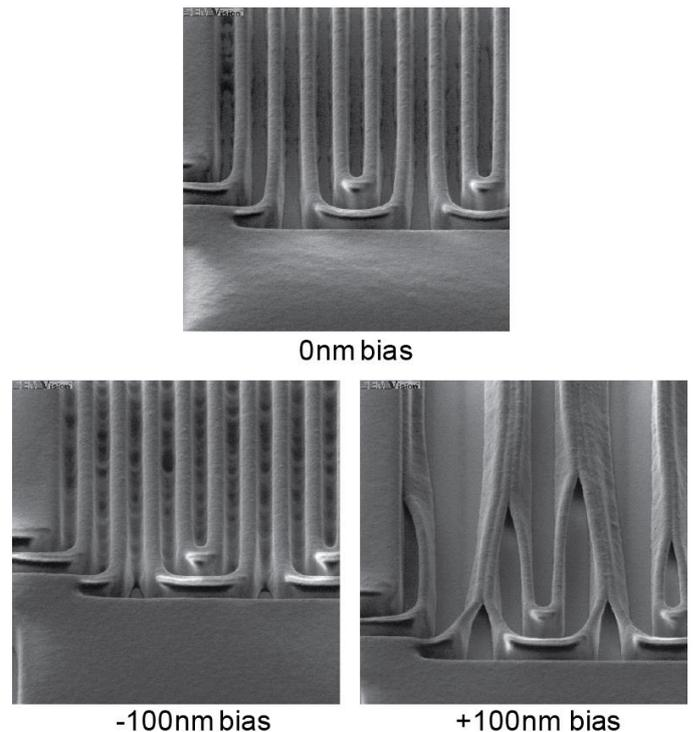
**Fig. 9:** Pattern fidelity of 1  $\mu$ m line/space meandercomb in photosensitive dielectric after full cure as a function of bias shows sensitivity to CD change.
