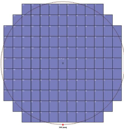
**Fig. 5:** Layout of 300 mm wafer with wafer edge protection used to clear the edge for electrical contact.
