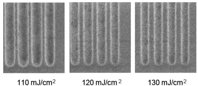
**Fig. 3:** Top down SEM images of 1μm line/space in 3μm thick JSR photosensitive dielectric on Si through exposure dose, i-line exposure, 0.20 NA.
