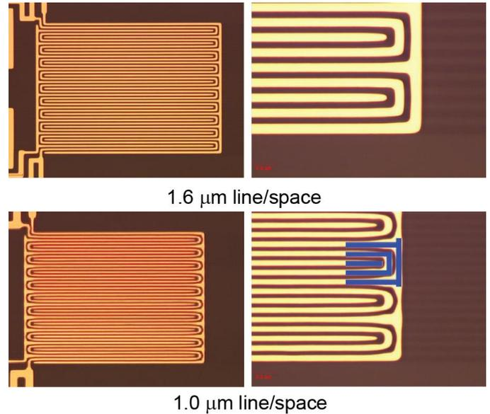
**Fig. 12:** Top images are of 1.6 $\mu\text{m}$  line/space meandercomb, and the bottom images are 1.0 $\mu\text{m}$  line/space meandercomb test structure after full CMP process. The blue inset represents design (ideal) pattern.
